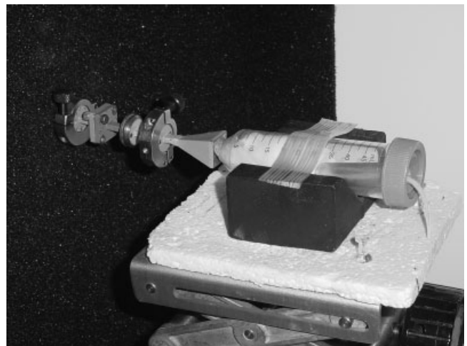
Fig. 1. Experimental set-up for irradiation of mice. For irradiation the animals were restrained in plastic tubes (3.5 cm diameter) with the nose uncovered for breathing and exposure purposes. Each mouse was positioned in such a way that its nose was placed in the center of the antenna aperture at a distance of 0–1 mm from its front edge.
